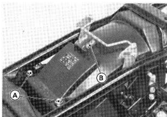
A. Upper Mounting Bolts B. Lock Lever Springs
